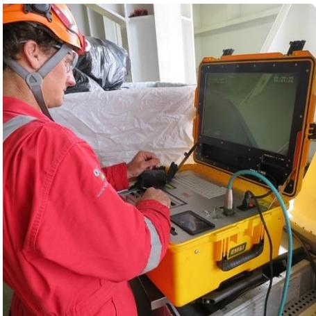
Controlled remotely, the NoMan confined space inspection unit enables thorough inspection without exposing personnel to hazardous environments. (Source: EM&I)
