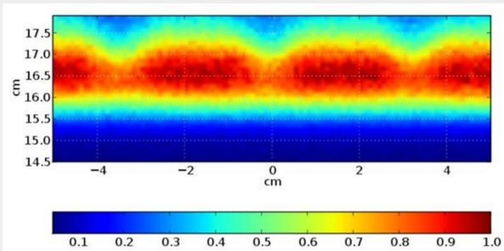
This BCT image shows the cross section of an insulated steel wall. Image courtesy of EM&I Stantec.
