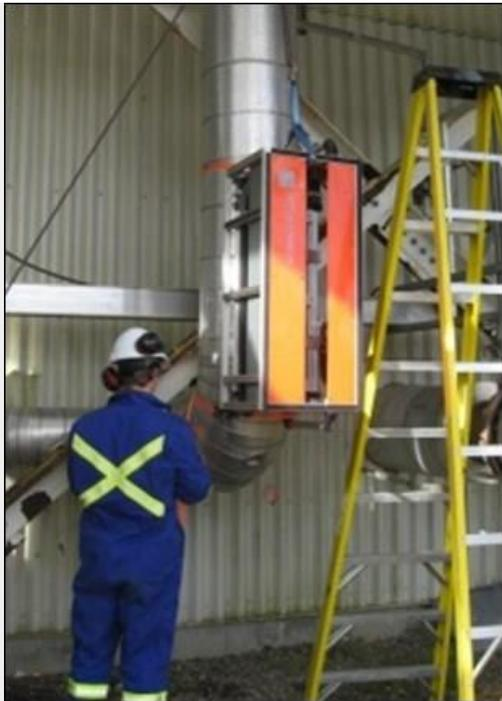
A BCT scanner, hoisted into place with an overhead line, is strapped to a 12-in (305-mm) insulated process gas line. Photo courtesy of EM&I Stantec and Inversa.
