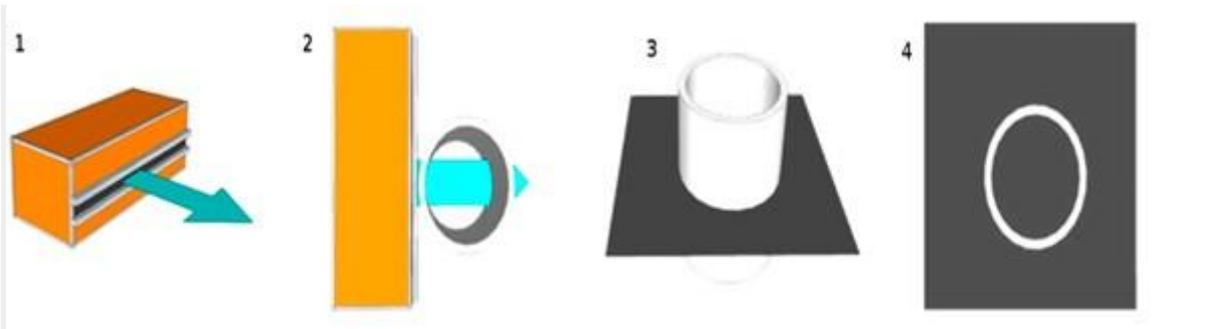
The illustration shows steps for creating a BCT scan. 1) The BCT scanner houses the radiation collimator and detector; 2) the scanner is placed adjacent to asset to be inspected; 3) data are collected for a single plane through the asset by measuring backscattered radiation; 4) measurements are numerically processed (reconstructed) by a computer algorithm to create a cross-sectional image of the object's density. Image courtesy of EM&I Stantec.
