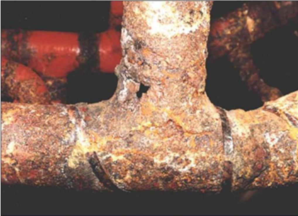
Typical pipe damage caused by CUI. Photo courtesy of EM&I Stantec.
