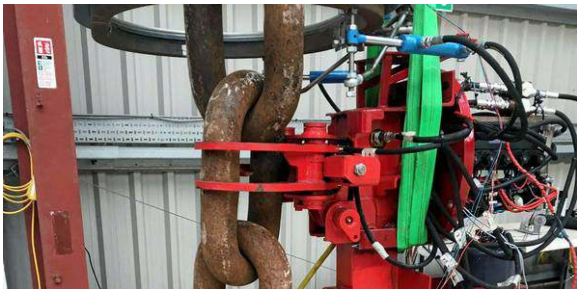
Grip: inspired, by the forestry sector, the 'LORIS' is used for inspecting mooring chains Photo: EM&I
