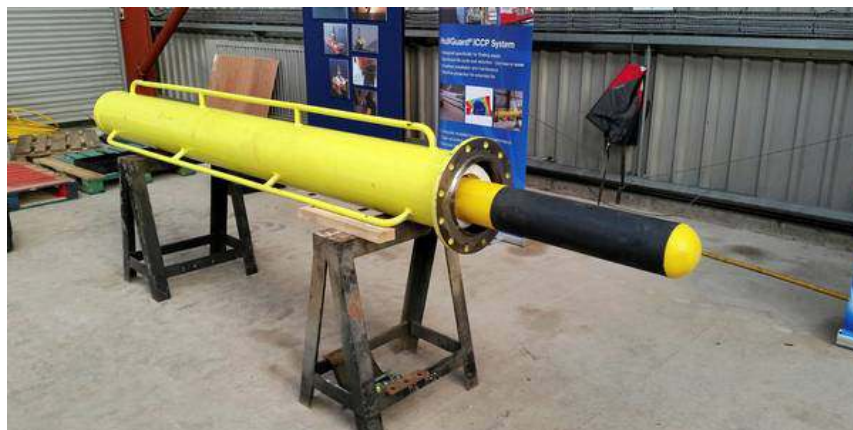
Innovation: An EM&I retractable anode removes the need for diver or ROV maintenance Photo: EM&I
