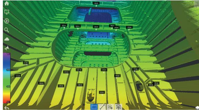
The NoMan technology enables the insertion of lasers into class-approved deck openings, to scan tanks to check for any degradation
