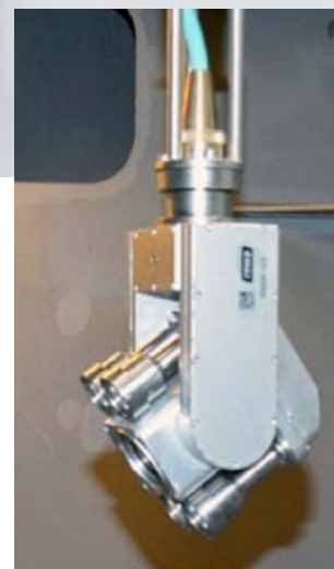
Remote camera inspection.
